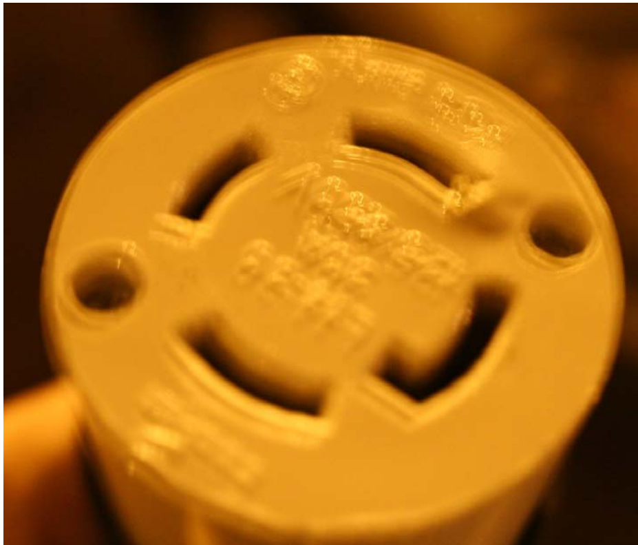
Original 220 VAC Charging Connector, Vehicle Side
